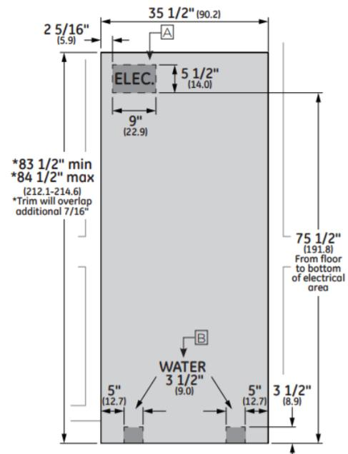
\* Shipping height. Use leveling legs and wheels for maximum 1" height adjustment from shipping height.
