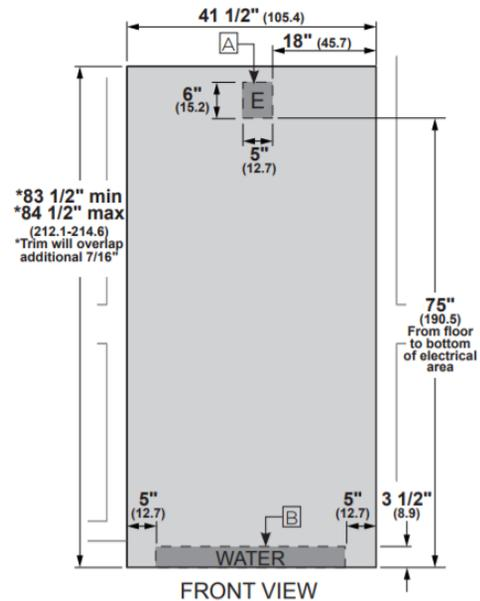
\* Shipping height. Use leveling legs and wheels for maximum 1" height adjustment from shipping height.
