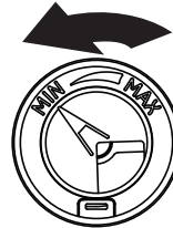
Counterclockwise to reduce foaming
