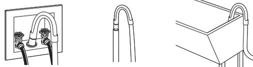
**NOTE:** If the drain hose is placed in a standpipe without forming a U shape, a siphoning action could occur. There must be an air gap around the drain hose. A snug hose fit can also cause a siphoning action.
