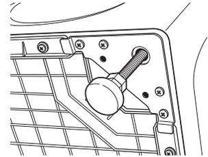
to ensure the washer is resting solid. Turn the lock nuts on each leg up towards the base of the washer and snug with a wrench.
