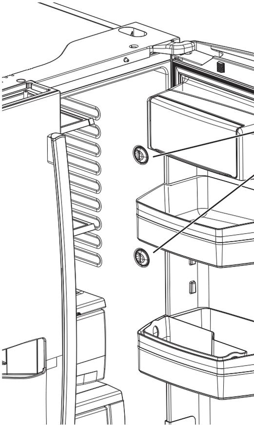
There is LED lighting in fresh food compartment and on the bottom of the fresh food doors to light the freezer compartment.\*
