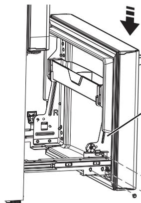
Align and insert tab on Freezer Door Bracket with slot on Freezer Slide Bracket.
