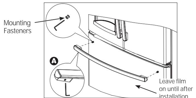
Reinstall the handles using the same procedure as removing.
