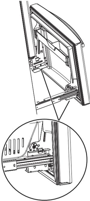
**A** Locate the height adjuster cam in the freezer door. Slightly loosen the three door attachment screws on both sides using a 3/8" hex socket driver.
