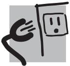
**Do not, under any circumstances, cut or remove the third (ground) prong from the power cord. For personal safety, this appliance must be properly grounded.**
