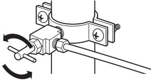
Turn the water on at the shutoff valve (house water supply) and check for any leaks.
