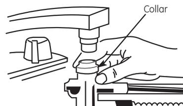
**Note:** The unicumple's small hose carries water from the faucet to the dishwasher. The large hose carries water from the dishwasher to the sink. Orient the faucet with the unicumple attached so water from the unicumple will run into the sink drain.
