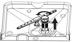
STEP 1: Turn the filter counter-clockwise and lift up.
