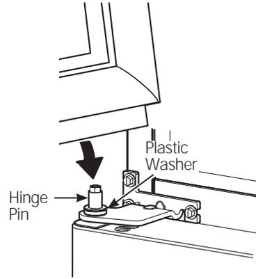
6.2.2 Tilt the door towards the cabinet, lifting the top hinge so the pin fits into the socket on the top of the door.
