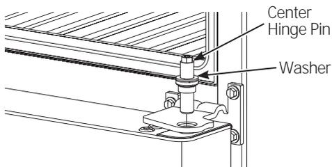
3.3 Remove the tape and tilt the door away from the cabinet. Lift the door from the pin in the bottom hinge. (If the plastic washer sticks to the door bottom, put it back on the hinge.)
