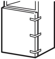
3.2 Unscrew the center hinge pin and remove it from its socket. Be careful not to lose the center hinge and washer.
