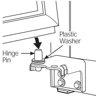
6.1.2 Tilt the door towards the cabinet. As the door is brought into position, align the socket in the door with the hole in the center hinge. Place the center hinge pin into the hole in the center hinge and tighten. Make sure the washer is on the top of the hinge pin.
