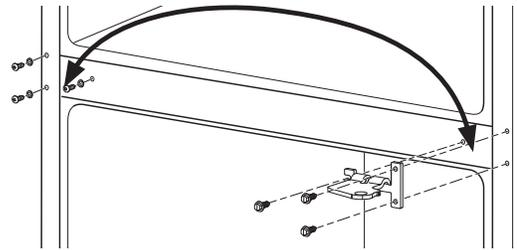
4.4 Reattach the center hinge with all three screws on the left side of the cabinet. **NOTE:** The center hinge must be turned over as shown when mounted on the left side.
