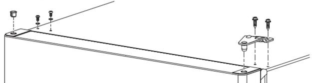
4.2 Remove the three screws holding the center hinge to the cabinet.
