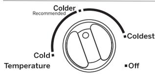
The temperature control adjusts the refrigerator from its warmest to coldest settings. Your refrigerator will come with the recommended factory setting on "Colder". For colder temperature, turn the knob clockwise to setting "Coldest". For warmer temperature, turn the dial counter-clockwise to setting "Cold". To turn off the cooling in both compartments, turn the knob clockwise to setting "Off". Note that this does not shut off power to the refrigerator.
