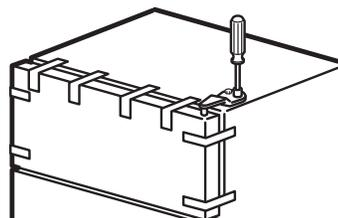
2.3 Lift the hinge straight up to free the hinge pin from the socket in the top of the door and set it aside, along with its screws.
