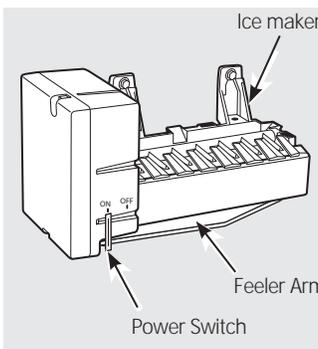
**CAUTION** Avoid contact with the moving parts of the ejector mechanism, or with the heating element (located on the bottom of the ice maker) that releases the cubes. Do not place fingers or hands on the automatic ice making mechanism while the refrigerator is plugged in.
