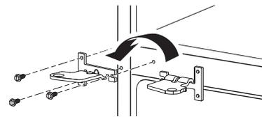
4.5 Remove the screws holding the bottom hinge to the cabinet. Move the bottom hinge from the right to left side of the cabinet. Switch the hinge pin to the opposite side of the hinge and reinsert the screws.
