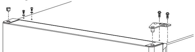
4.2 Remove the three screws holding the center hinge to the cabinet.
