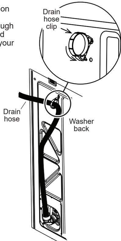
If water valves and drain are built into wall, fasten drain hose to one of the water hoses with cable tie provided.
