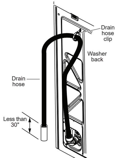
**NOTE: Placing the drain hose too far down the drain pipe can cause a siphoning action. No more than 5" of hose should be in the drain pipe. There must be an air gap around the drain hose. A snug fit can also cause a siphoning action.**
