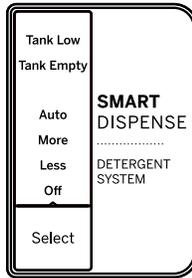
If it is desired to manually select the amount of detergent for a given load, this can be done by pressing the **Select**
