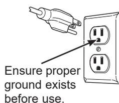
Washer must be electrically grounded in accordance with local codes and ordinances, or in the absence of local codes, with latest edition of the NATIONAL ELECTRICAL CODE, ANSI/NFPA NO. 70 or CANADIAN ELECTRICAL CODE, CSA C22.1. Check with a licensed electrician if you are not sure that the washer is properly grounded.
