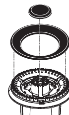
Multi-Ring Burner (on some models) Use this burner for large cookware or for simmering applications.
