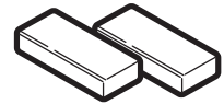
Filler blocks or scrap wood pieces, if needed for top cabinet spacing (used on recessed bottom cabinet installations only)
