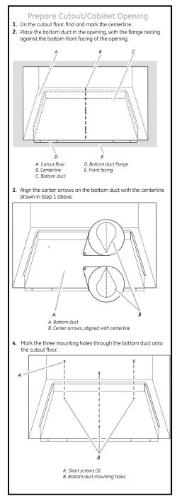
5. Using a 7/64" drill bit, drill pilot holes into the three hole marks shown in the figure above.
