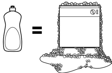
**NOTE:** Using a detergent that is not specifically designed for dishwashers will cause the dishwasher to fill with suds. During operation, these suds will spill out of the dishwasher vents, covering the kitchen floor and making the floor wet.
