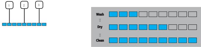
Located on the right side of the front of the dishwasher, these lights indicate how far along is the current wash cycle when the dishwasher is operation.
