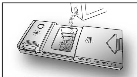
To open the wash cover, press the button and the cover will flip back.
