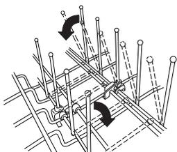
The fold down tines (on some models) provide flexibility for extra-large and hard-to-fit items. The tine rows can be adjusted to a vertical or lay-down position.
