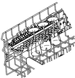
To add flexibility in loading, the utility shelf (on some models) may be placed in the up or down position. The shelf may also be used to secure stemware such as wine glasses. Because these stemware items come in various sizes, slowly push the rack in to ensure the items do not bump into the edges of the dishwasher, which may cause damage to the items.
