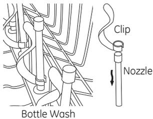
The **Bottle Wash** system is the ideal location to position baby bottles and tall sports bottles. The **Bottle Wash** clips hold bottles with small openings in place so water jets are directed inside the bottles to clean hard to reach areas. Clips can be installed or removed by simply slipping the clip opening over the top of the nozzle.
