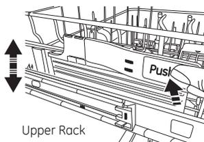
The upper rack allows 2" of adjustment up or down to accommodate large items. The upper rack may be lowered by pushing the long flaps on each side of the rack. This will allow you to lower the rack (see fig. Upper Rack). To raise the rack, lift up on the rack until the rack locks in place.
