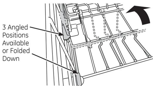
The **reversible tine blocks** are designed to allow greater flexibility in loading dishes. The direction of the tine blocks can be changed to match your preferred loading direction as shown in Figure A or Figure B.
