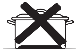
Pans with rounded, curved, ridged or warped bottoms are not recommended.
