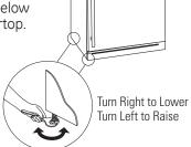
1/8" less than the opening height. Screw front legs all the way in to shorten the height at the front. This will allow you to slightly tip the unit into the opening. Once in the correct position, the front legs can be adjusted to level the product.
