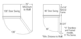
Allow 25" (63.5 cm) minimum clearance for a full 130° door swing. Allow 15" (38.0 cm) for pan removal.
