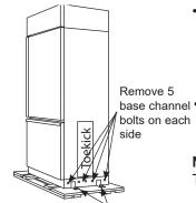
• The unit is secured to the skid with 4 slotted tie-down straps. Remove the six 7/16" bolts from the base channels in the tie-downs.
