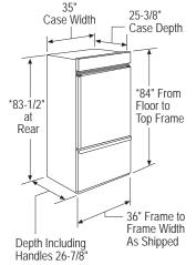
\* Shipping height. The refrigerator can be adjusted to fit into a cutout that is 84-1/2" (214.63 cm) max. height. Note that the top case trim at the front is 1/2" (1.27 cm) higher and will overlap upper cabinetry or soffit. Use leveling legs and wheels for a maximum 1" (2.54 cm) height adjustment.
