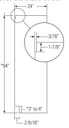
• Cut a notch in the top front corner as shown to allow clearance for corner keys in the front side trim.
