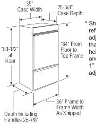
Shipping height. The refrigerator can be adjusted to fit into a cutout that is 85" (215.9 cm) max. height. Use leveling legs and wheels for a maximum 1" (2.54 cm) height adjustment.
