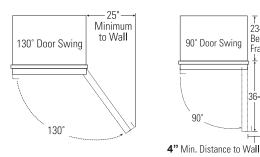
Allow 25" (63.5 cm) minimum clearance for a full 130° door swing. Allow 15" (38.1 cm) for pan removal.
