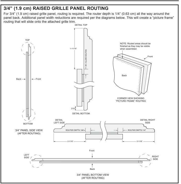
NOTE: For panels constructed with rails and stiles (5-panel), the minimum width is 3" (7.62 cm) for rails and 4" (10.16 cm) for stiles.
