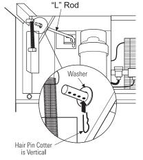
washer on the rod. Reinsert the pin.
