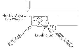
Adjust height of unit to match installation cutout opening 84-1/2" (214.63 cm). The unit should be level and plumb with cabinetry.
