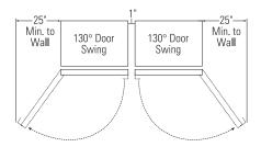
Clearances for Multiple Single Door Installations In a side-by-side installation of a left and right door swing product, a 1" (2.54 cm) clearance between the units is required. Order ZUGSS2 Stainless Steel Unified Grille Panel Kit or ZUG2 Custom Panel Unified Grille Panel Kit for one continuous grille panel.
