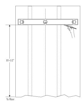
Place the bottom of the wall bracket with tabs on the horizontal line. Align the center notch on the bracket with the center line on the wall.
