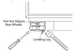
The rear leveling wheels and front leveling legs are limited to a maximum height adjustment of 1" (2.54 cm). If the installation requires more than 84-1/2" (214.63 cm) height, the installer should elevate the unit on a sheet of plywood or runners. Cabinetry trim could also be added across the top of the opening to shorten the opening. If you attempt to raise the unit more than 1" (2.54 cm), you will damage the front leveling legs and the rear leveling wheels.
