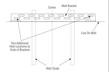
Mark an additional hole at each end of the bracket.
