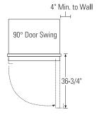
These units are equipped with a 3-position door stop. The factory set 115° door swing can be adjusted to 90° or 130° if clearance to adjacent cabinets or walls is restricted. Order WX14X99 door stop for precise settings between 90° and 130°.
