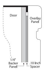
**NOTE:** Left-to-right offset is not always equal to top-to-bottom offset.
