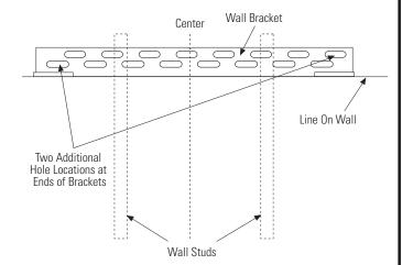
The anti-tip wall bracket has a series of holes. Select 2
