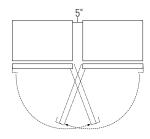
Clearances for two products installed side-byside with right and left side hinges together Allow 5" (12.7 cm) minimum between the two products to prevent one door from striking the other. Use the WX14X99 adjustable door stop to reduce the factory set 115° door swing and to allow pan removal.
