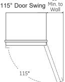
Allow 25" (63.5 cm) minimum clearance for a full 130° door swing. Allow 15" (38.1cm) for pan removal.
