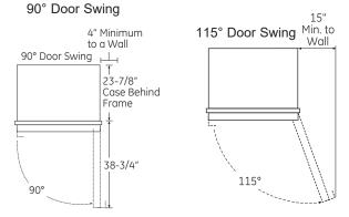
For a 90° door swing, allow 4" (10.16 cm) minimum clearance to a wall for framed and stainless steel models. If the 90° doorstop position is used, pan access is maintained but pan removal is restricted.
