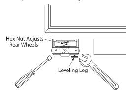
The rear leveling wheels and front leveling legs are limited to a maximum height adjustment of 1" (2.54 cm). If the installation requires more than 84-1/2" (214.63 cm) height, the installer should elevate the unit on a sheet of plywood or runners. Cabinetry trim could also be added across the top of the opening to shorten the opening. If you attempt to raise the unit more than 1" (2.54 cm), you will damage the front leveling legs and the rear leveling wheels.
