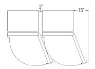
Clearances for two products installed side-by-side with the same (left or right) door swing Allow 2" (5.08 cm) minimum clearance between the products to prevent door swing interference. Order the WX14X99 adjustable door stop to reduce the factory set 115° door swing. Allow 15" (38.1cm) minimum to a wall to achieve full drawer extension and pan removal.
