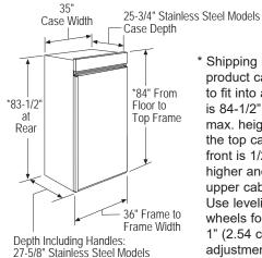
\* Shipping height. The product can be adjusted to fit into a cutout that is 84-1/2" (214.63 cm) max. height. Note that the top case trim at the front is 1/2" (1.27 cm) higher and will overlap upper cabinetry or soffit. Use leveling legs and wheels for a maximum 1" (2.54 cm) height adjustment.
