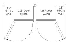
Clearances for Multiple Single Door Installations In a side-by-side installation of a left and right door swing product, a 1" (2.54 cm) clearance between the units is required. Order ZUG2 Unified Grille Panel Kit for one continuous grille panel.
