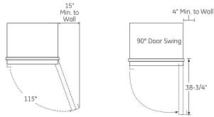
These units are equipped with a 3-position door stop. The factory set 115° door swing can be adjusted to 90° if clearance to adjacent cabinets or walls is restricted.
