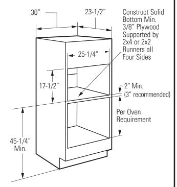
• If you are replacing a GE/Monogram electric double oven with the combined installation of an Advantium 240V and a single oven, use the dimensions shown. The middle rail separating the two openings may need to be larger than the 2" minimum shown.
