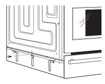
Place the side supports into the tabs on the drawer and secure using the screws supplied and the screws removed in Step C.
