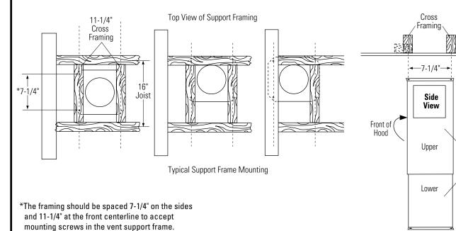
IMPORTANT: The cross framing must be spaced 7-1/4" from centerline to centerline in order to accept the hood
