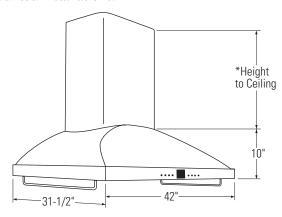
\* 20" to an 8 ft. ceiling. Using supplied duct cover
