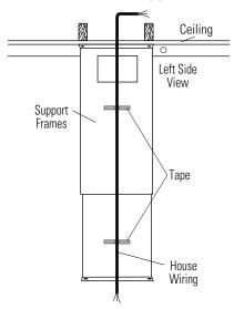
• Tape the wire to the left side of the frame support to prevent damage during installation and service.
