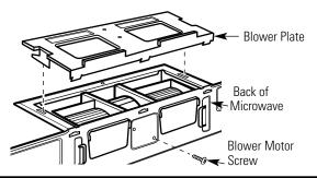
**5** Carefully pull out the blower unit. The wires will extend far enough to allow you to adjust the blower unit.
