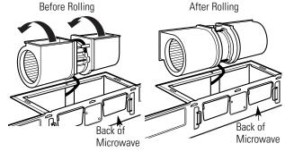
4 Gently slip the wire through the gap between the two tabs on the top of the blower so the wire is behind the tabs.
