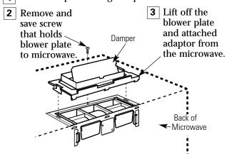
4 Slide exhaust adaptor to one side and remove it.
