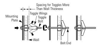
**3** Place the mounting plate against the wall and insert the toggle wings into the holes in the wall to mount the plate.
