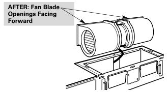
7 Place the blower unit back into the opening. CAUTION: Do not pull or stretch the blower unit wiring. Make sure the wires are not pinched.
