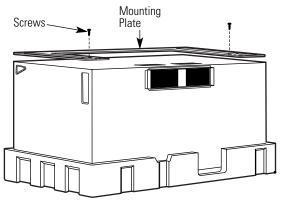
Remove the 2 screws from the mounting plate.
