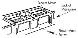
2 Carefully pull out the blower unit. The wires will extend far enough to allow you to adjust the blower unit.
