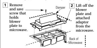
3 Slide exhaust adaptor to one side and remove it. **NOTE:** The exhaust adaptor with damper is not needed for recirculating models. You may want to save them for possible future use.
